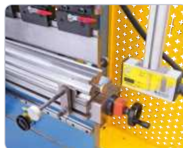
Serially with manual table crowning system with digital readout.
