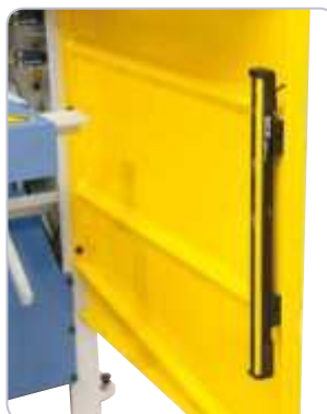
Sick-light barrier on the backside of the machine (optional)
