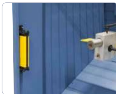
The standard light barrier prevents intervention in the running machine.
