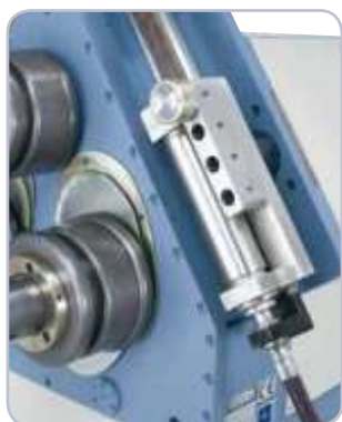
Illustration BPK 80 H with hydraulically adjustable guiding rolls in 2 directions (option).
