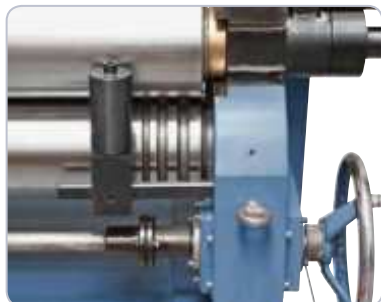
Bottom and back roller with wire insert groove
