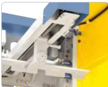
Backgauge with ball screw for increased accuracy.
