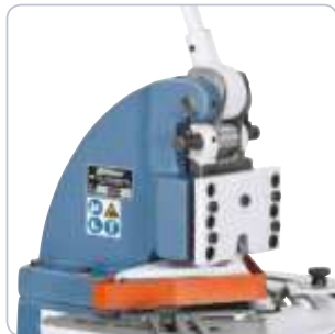
Mechanical power transmission by means of eccentric.
