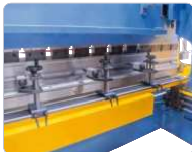
3 pcs. height-adjustable backgauge fingers, laterally adjustable via linear guide
