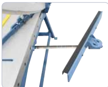
Adjustable backgauge for extended application.
