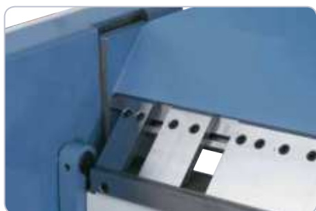
The removable segments allow a variety of bending options.
