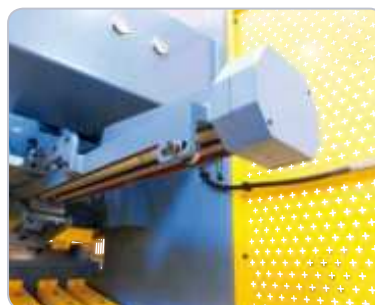
Backgauge with ball screw for increased accuracy.
