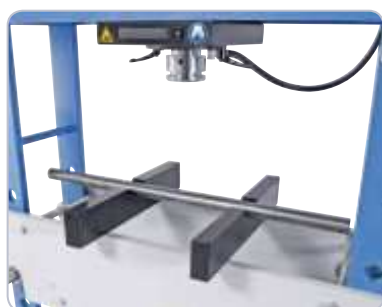
For straightening shafts, optional prism supports are available.
