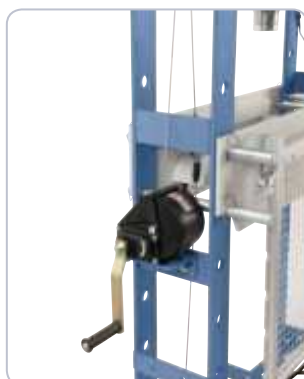
Integrated winch for easy height adjustment of the support table.
