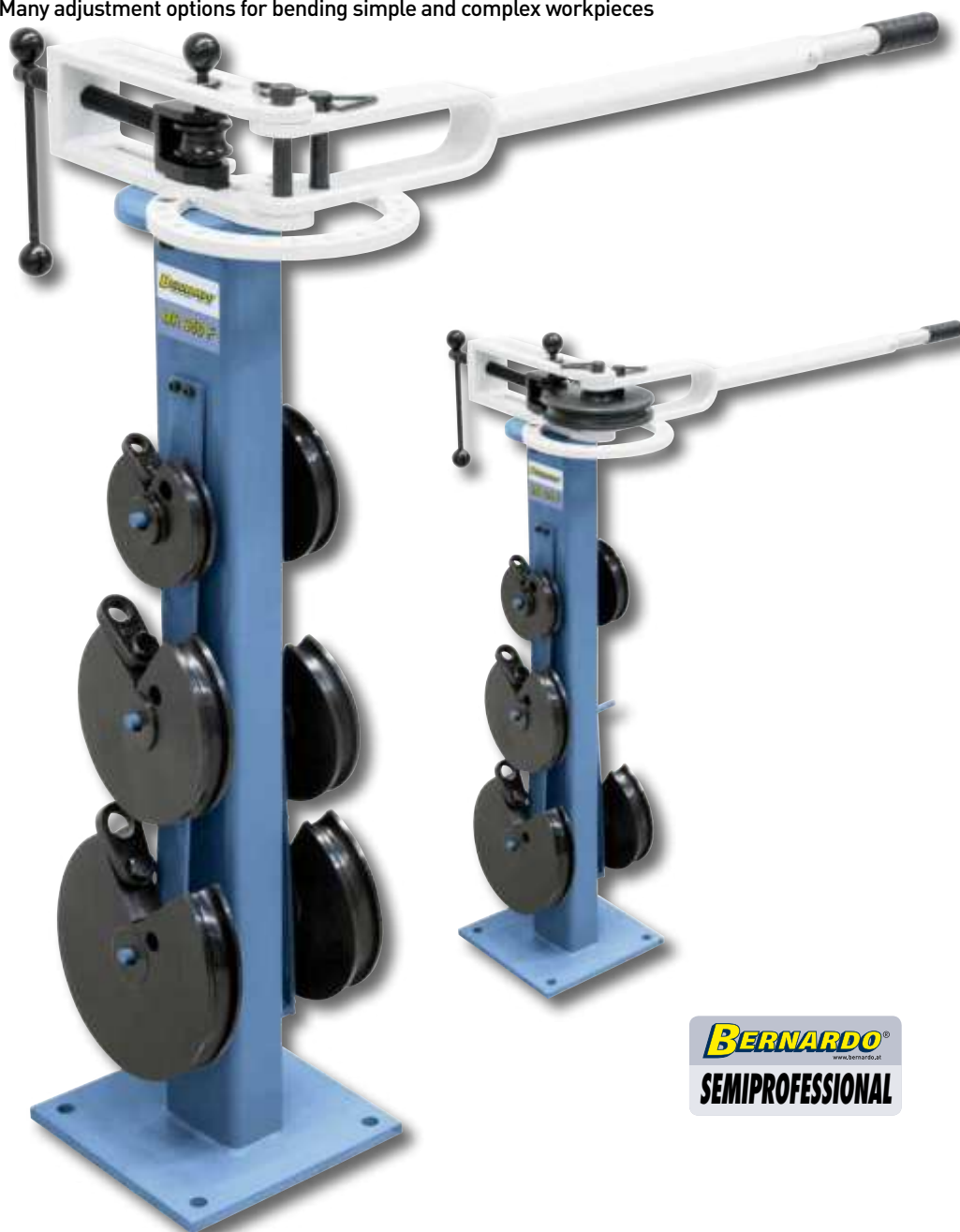
High repeatability due to the bending angle stop
