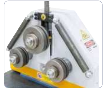
The lateral guiding rolls can be steplessly adjusted to the respective profile.
