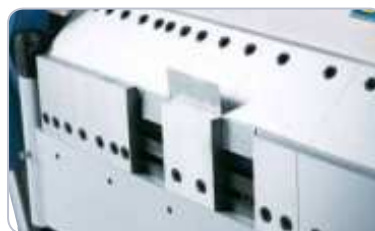
Due to the segmented bending beam also opposite bends can be performed.
