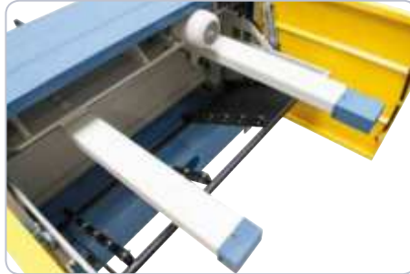
Pneumatic sheet support system, the user can optionally set the sheet ejection to the operator side or back of the machine.
