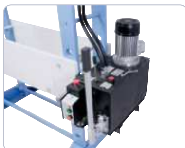
The piston stroke takes place alternatively by hand lever or hydraulic pump.
