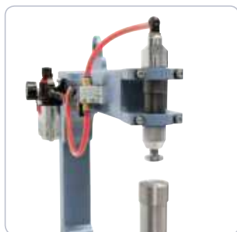
Punching dies exchangeable within seconds.
