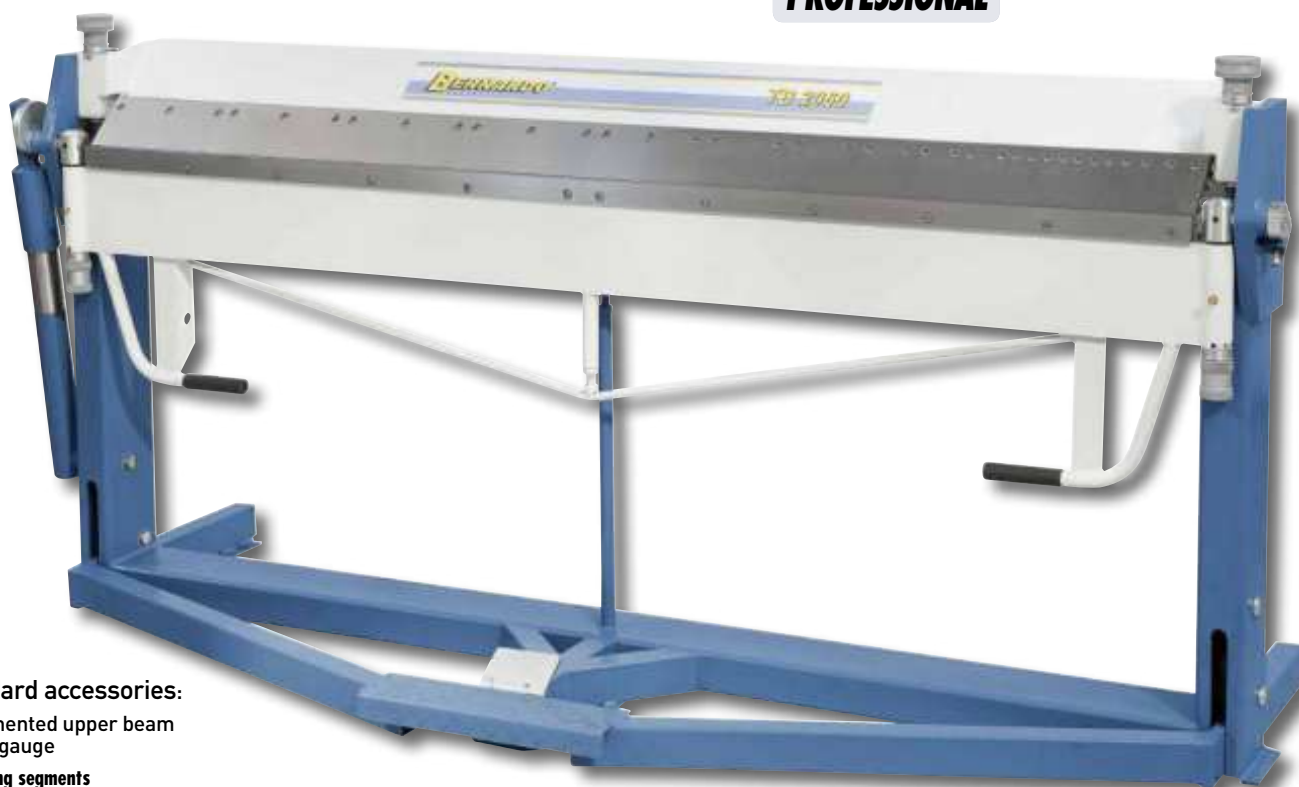
Hardened and ground segments ensure precise bending.
