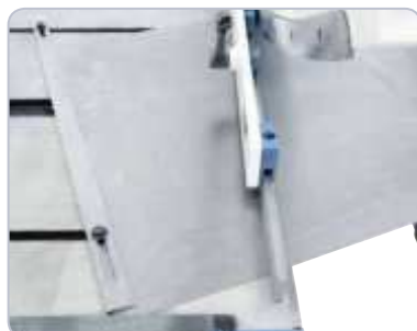
Precise work results through table fence and downholder.
