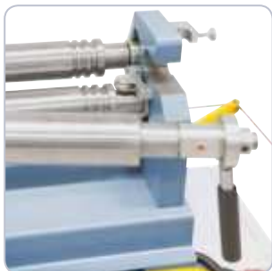
Forward swivelling upper roller for easy removal of the finished workpiece.
