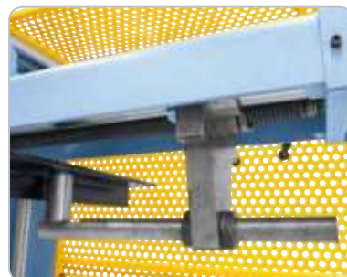
Serially with motorized backgauge up to 750 mm.
