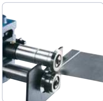
Example of use: connecting beads
