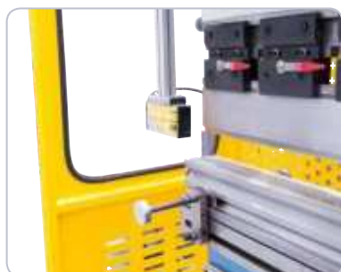
Non-contact, moving, laser-optical safety system Fissler AKAS-LC II.
