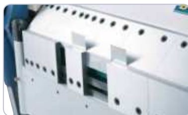
Due to the segmented bending beam also opposite bends can be performed.
