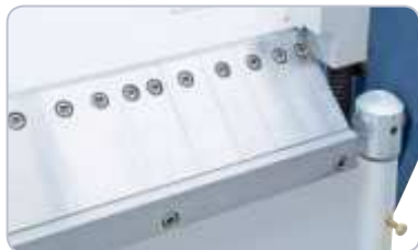
Hardened and ground segments ensure precise bending.
