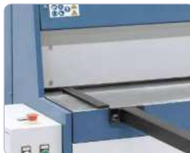
Exact, right-angled adjustment by lateral stop.
