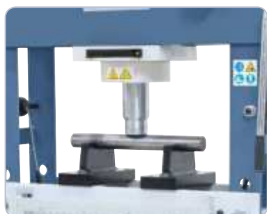
Standard with support prism for straightening of shafts.
