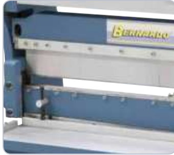
The removable inserts result in a high number of bending possibilities.
