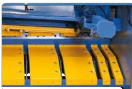
The pneumatic sheet support system (standard) prevents the bending of thin sheets and therefore ensures an exact cut.
