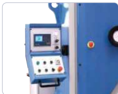
Integrated control NC 10 in the control panel, standard with memory function
