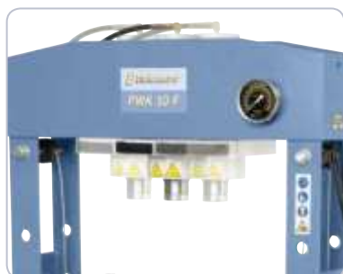
Movable pressure cylinder for universal use.
