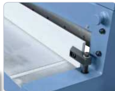
Inlaid measuring tapes in the work table.
