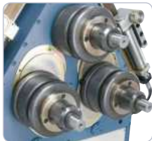
Hardened and ground rolls and shafts.
