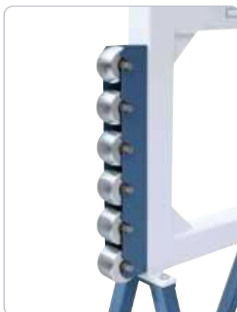
Practical holder for the anvil wheels on the side of the machine body.
