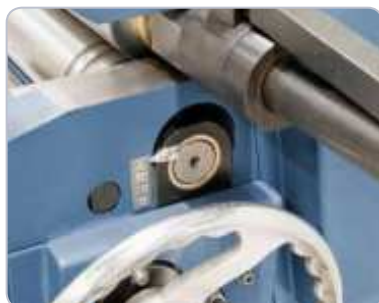
Exact adjustment of the bottom roll by scale.
