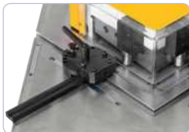
The T-slots in the work table provide precise guidance of the stops.
