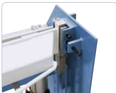
Optimal guidance of the upper knife through robust rectangular guide
