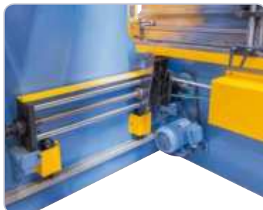
Backgauge serially with ball screw for increased accuracy.
