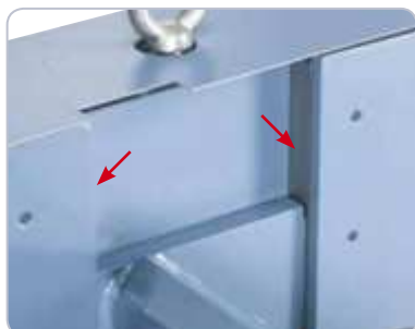
Large dimensioned guide guarantees exact bending.
