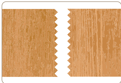
Prong bonding of boards guarantees high rigidity and maximum strength
