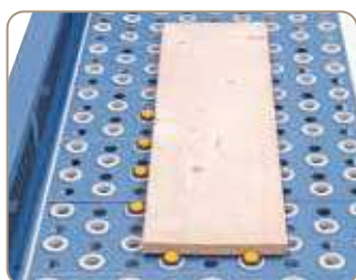
Standard with stops for positioning the workpiece.
