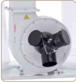
Comes complete with dust port to use three machines at the same time.
