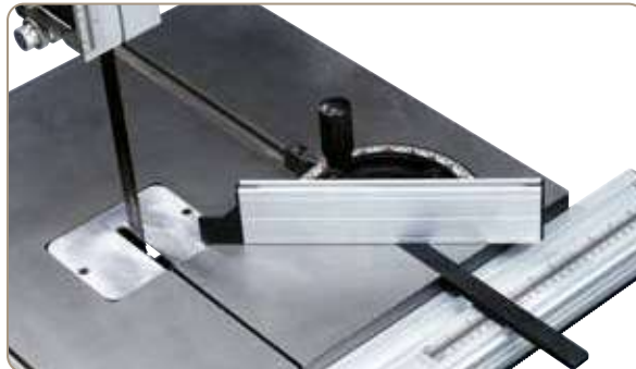
Amply sized working table with grounded surface and T-slot for the mitre fence (standard)
