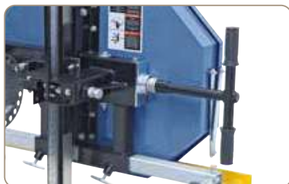
User-friendly tensioning of bandsaw blade, easy to access.
