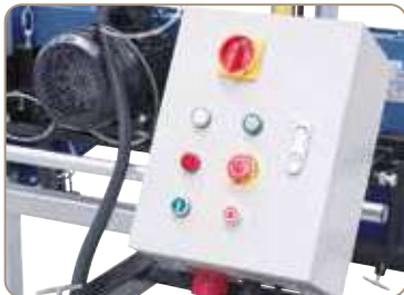
Picture shows electronic panel and push stick for manual feed (height adjustable).
