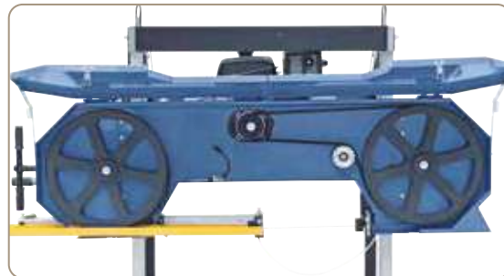
Tiltable covers allow for easy bandsaw blade change.
