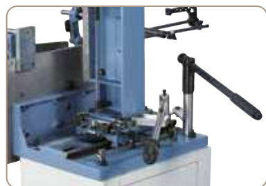
Cross and longitudinal movement feature adjustable fences.
