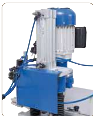
Maintenance-free aluminium feed cylinder.
