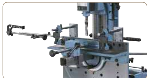
Solid work table tilts 45° to the right and left.
