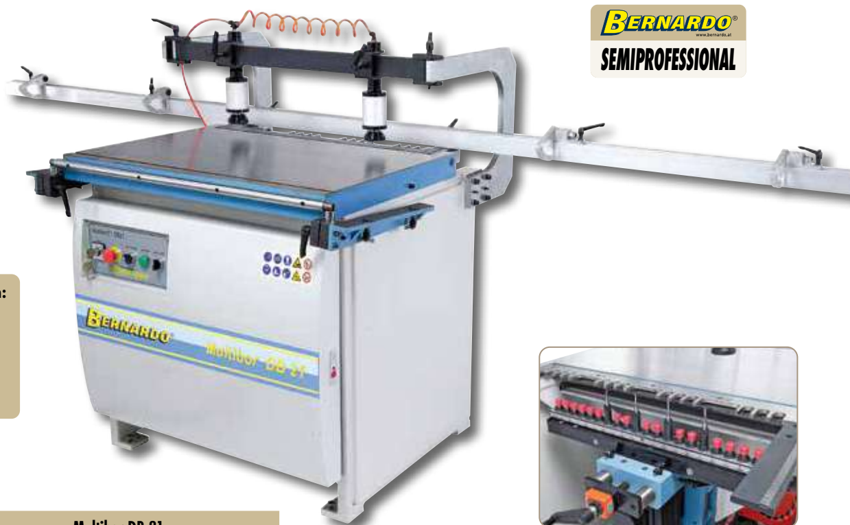
Fence with 3 gaps to use with multiple drill heads for hinges
