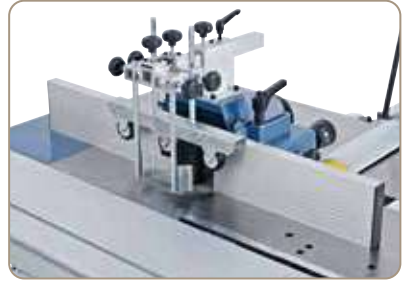
The moulding fence comes complete with fence rails made of anodized aluminium.
