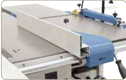
Tiltable parallel fence with micro-metric fine adjustment.
