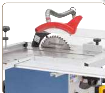
Protective sawblade cover with integrated dust port connected on riving knife.
