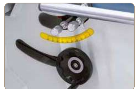
User-friendly height and side adjustment of scoring unit.
