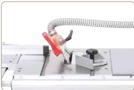
Left tilting sawblade enables workpiece to be guided more easily during cut.
