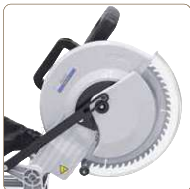
Sawblade gets covered automatically when lifting the sawblade
