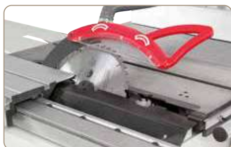
Sawblade cover, featuring integrated dust port, connected to riving knife. Standard equipment includes scoring unit.
