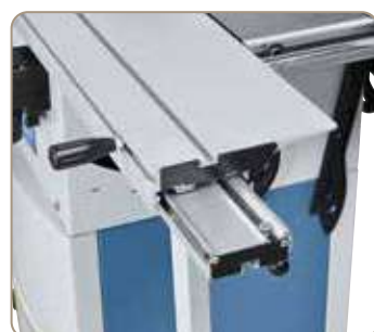
Hardened prism-shaped guide for smooth running of sliding table.
