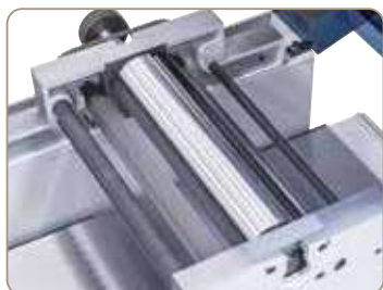
The precisely bedded 4-knife cutterblock and the straight-toothed of the infeed roller ensure top work results.
