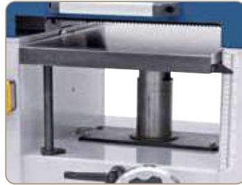
The torsion-free thickening table is guided on a central column with support.
