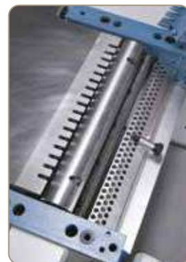
The table lips in combination with the perforated chip plate keep the noise level to a minimum.
