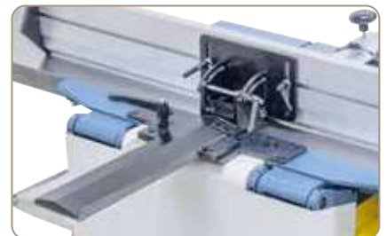
The planer fence can be set to required position via the precise prism guide.
