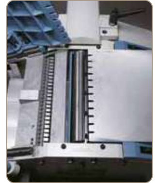
The precisely bedded cutterblock and corrugated infeed roller guarantees best planing results.
