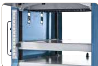
Thicknessing table on four guides, height adjustable on clearly designed scale.
