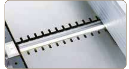
The planing tables are designed with slots to keep noise levels to a minimum.
